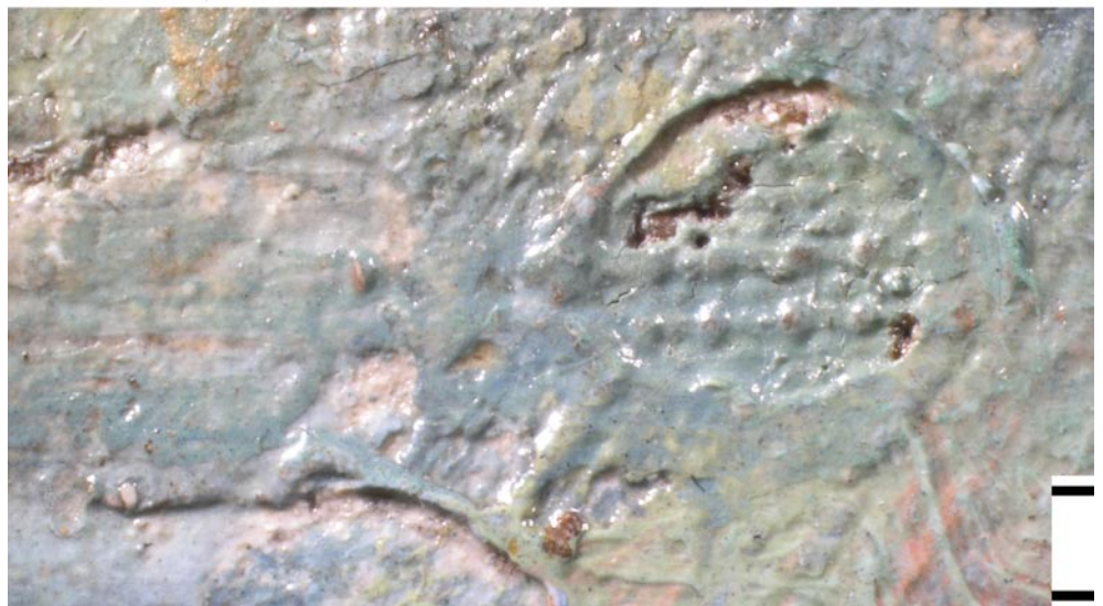
Fig. 12 Left-hand corner, circular impressions in the fresh paint-layer presumably resulting from commercial spacers (see above), microscopic photograph (M = 1 mm)
