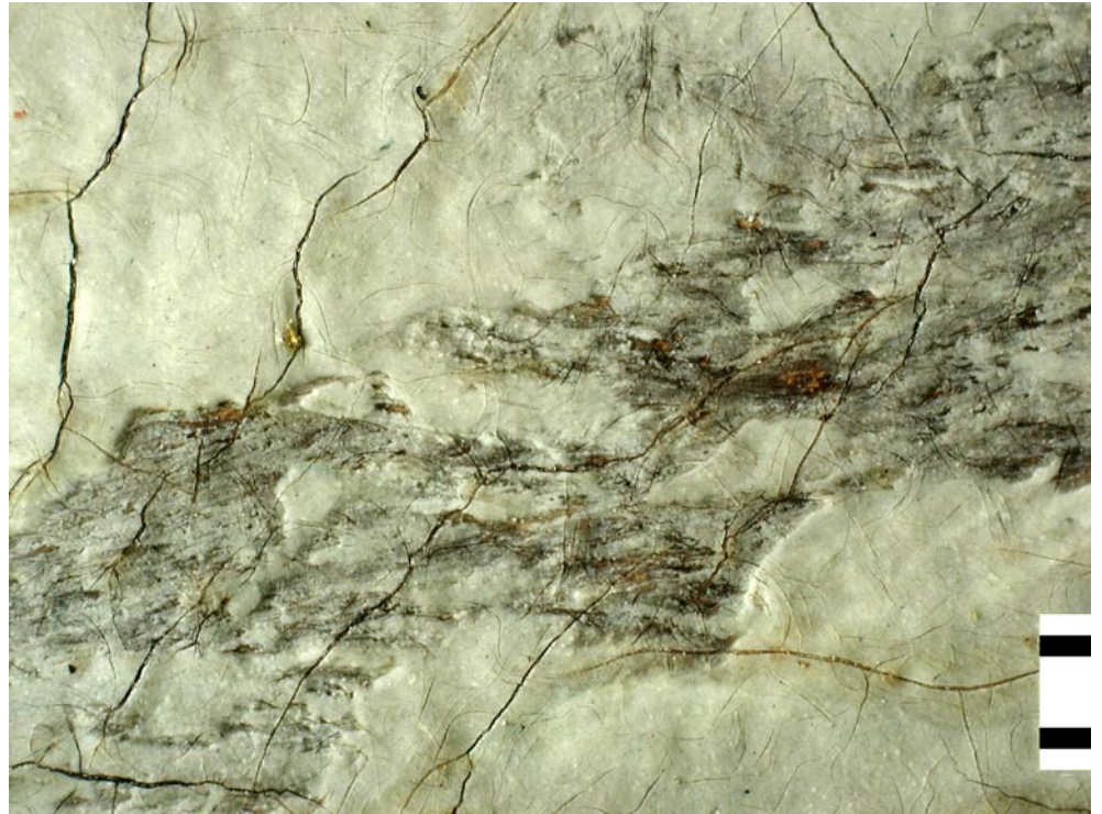
Fig. 11 Scratches in light-grey paint layer in the clouds, microscopic photograph (M = 1 mm)
