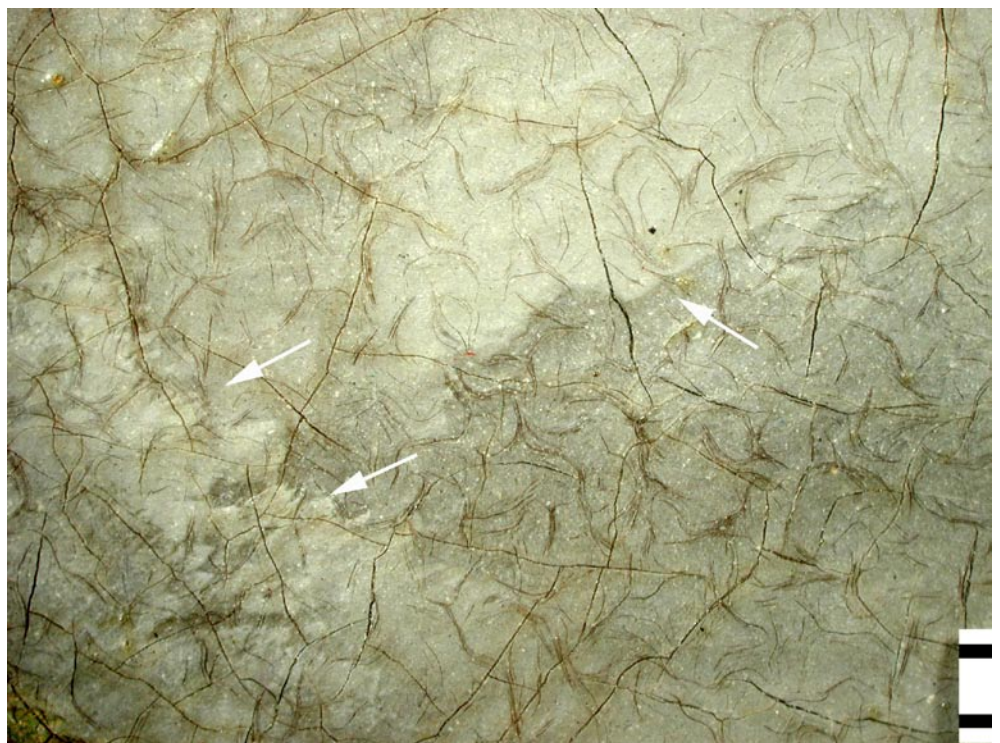
Fig. 10 Trowel and brush application (arrows), typical fine craquelure, microscopic photograph (M = 1 mm)
