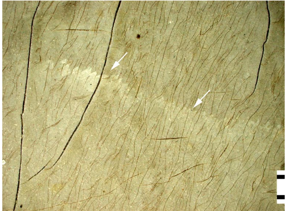
Fig. 9 Glazed thin paint application (arrows), microscopic photograph (M = 1 mm)
