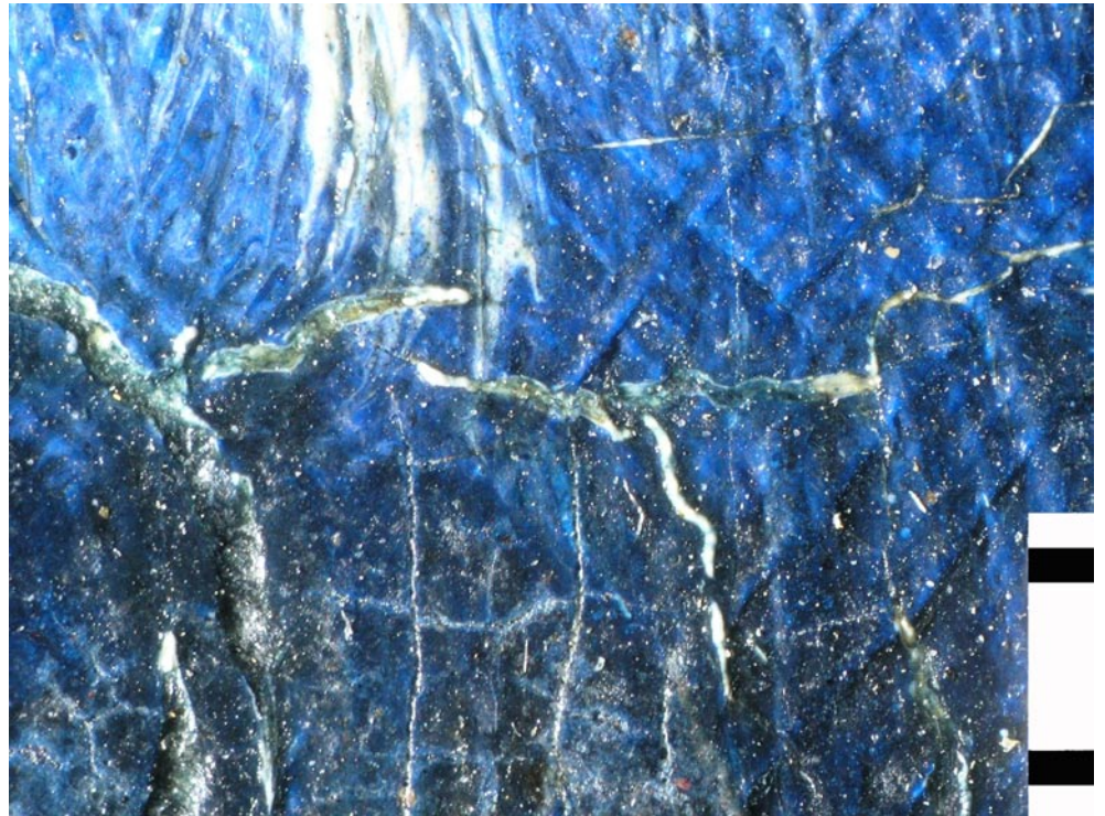
Fig. 9 Early shrinkage cracks in the intermediate coat have been partially retouched during a restoration which cannot be dated, microscopic photograph (M = 1 mm)
