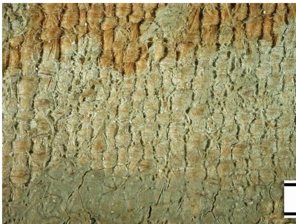
Fig. 10 Edge of the ground on the turnover edge; the pale, thin layer that barely fills the pores is followed by the actual grey-green ground itself, microscopic photograph (M = 1 mm)
