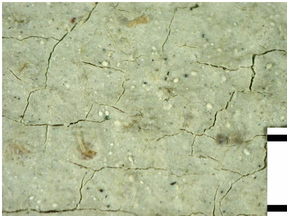
Fig. 9 Grey-green ground with conspicuously coarse white pigments, microscopic photograph (M = 1 mm)
