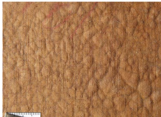
Fig. 13 Details, raking light photographs of the canvas recto and verso show cleavage and deformations of the canvas, which have been caused by the raising of individual patches of the paint layer
