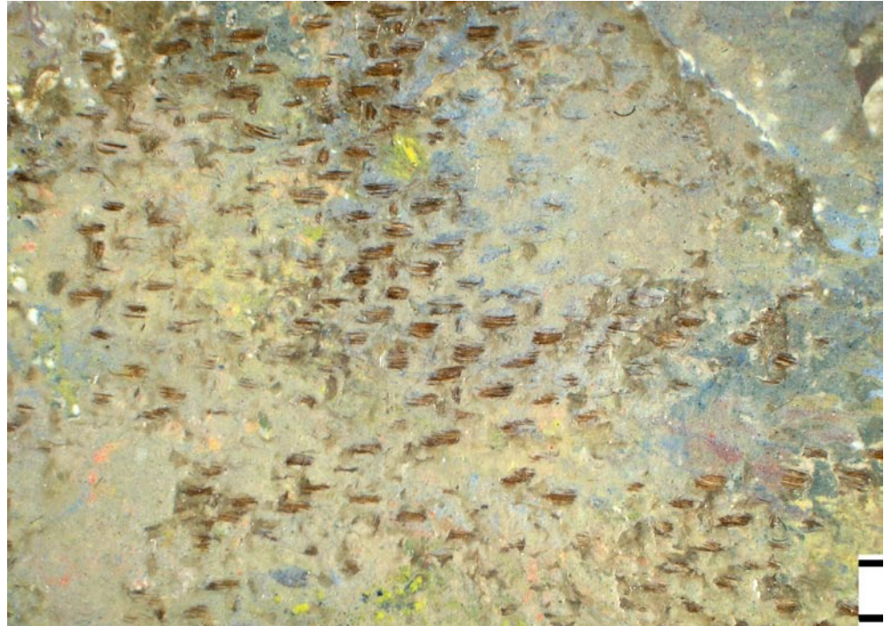
Fig. 13 Abrasions of the paint-layer and ground right down to the canvas, due to inexpert varnish removal or surface cleaning, microscopic photograph (M = 1 mm)
