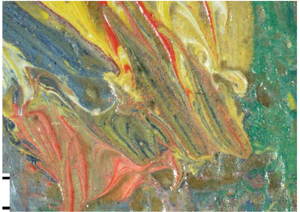
Fig. 11 Paints of various colours applied wet-in-wet blending in the brush- stroke, microscopic photograph (M = 1 mm)
