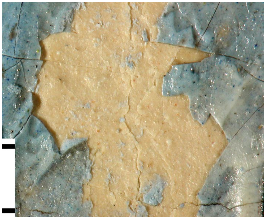
Fig. 8 Cream ground, microscopic photograph (M = 1 mm)
